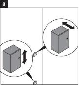
Check the scews which allow adjustments of the unit.
