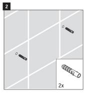
Drill the anchor holes that have been marked. The Plastic anchors provided are for concrete wall applications. Insert plastic anchors into the holes.
