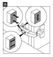
The top screw will adjust up and down. Back screw will adjust closer and further. From the cabinet and front screw will adjust left and right.
