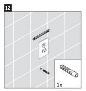
The plastic anchor provided is for concrete wall applications.
