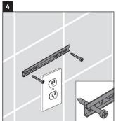
Screw the bracket(s) to the wall at the specified locations. For wood stud walls, bolts should be screwed into the wood backing.
