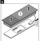
Lift the mirror up and slide the mirror backing.
