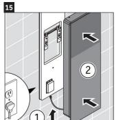
Plug the unit into the outlet, plug the cord(1) into control unit. Slide the unit onto the mirror backing.
