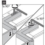
Using allen wrench, tighten the top middle screw clockwise one turn 90 degree or counter-clockwise one turn 90 degree until desired leveling of the hinged mirror has been reached.
