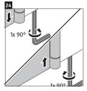
Using allen wrench tighten screw counter-clockwise one turn 90 degree or clockwise one turn 90 degree until desired leveling of the hinged mirror has been reached.
