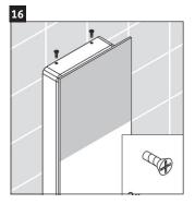
Attach mirror front to mirror backing with two top supplied screws.
