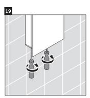
Using a screwdriver tighten the screws clockwise.
