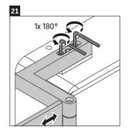
Using allen wrench, tighten the top screws clockwise one turn 180 degree.
