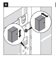
The top screw will adjust closer and further, from the mirror and lower screw will adjust up and down.
