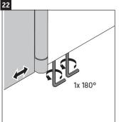
Using allen wrench tighten the bottom screws counterclockwise one turn 180 degree.
