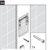
Screw the bolt to the wall at the specified location. For wood stud walls, bolts should be screwed into wood backing.
