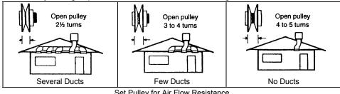
Set Pulley for Air Flow Resistance (Figure 7)
