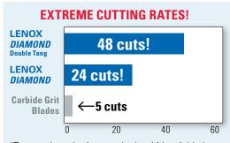
\*Test conducted using standard carbide grit blades vs. 11" LENOX DIAMOND Double Tang cutting 2" cast iron pipe in laboratory testing
