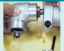
Quick switch drill head for low or high speed settings
