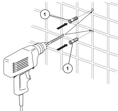
**NOTE:** If possible, it is best to mount at least one end of your towel bar into a wall stud. Try to locate a wall stud with a stud finder or by tapping on the wall. Place mounting bracket (1) in the desired location. Ensure the mounting bracket is level; then, mark the position of the holes (2) on the wall. Repeat for 2nd mounting bracket, spaced as noted above.
