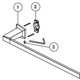
Position body (1) over mounting bracket (2) and tighten set screw (3). (Set screw should be on the bottom of body.) Place one end of the towel bar (4) into the second body (5), and place the other end of the bar into the first body (1). Slide the second body over the other mounting bracket (6) and tighten set screw (7).
