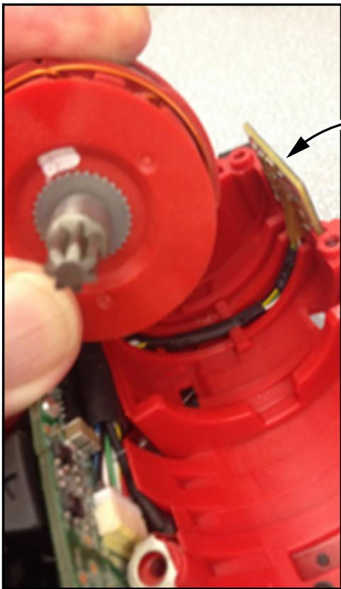
Prior to installing Stator/Rotor Assemblies, place the Selector PCBA into the slotted Housing Support cavity. Press wires into channel as shown. Carefully place Stator/Rotor Assemblies into Housing Support, being sure all components are firmly and squarely seated.
