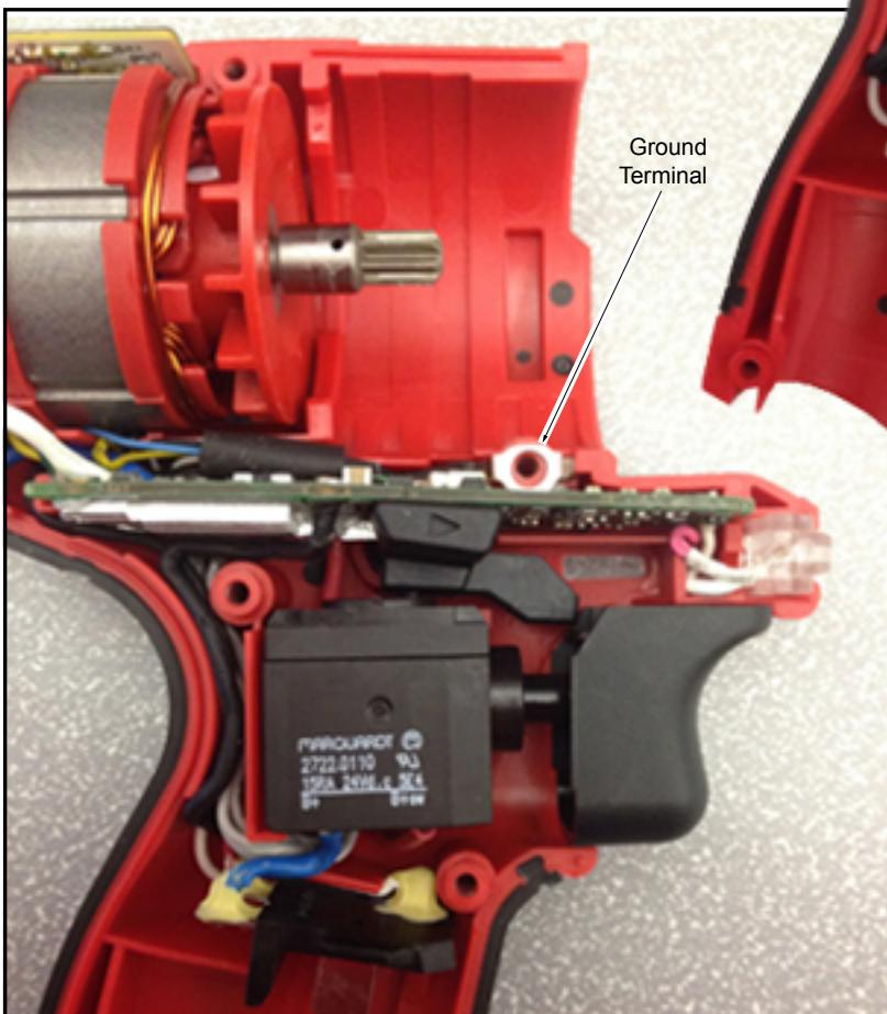
Prior to installing the Gear Case Assembly, be sure all elements of the Electronics Assembly are seated properly (Stator, Main PCBA, Selector PCBA, On-Off Switch, LED Assembly and Battery Terminal Block Connector). Be sure the Grounding Terminal is in place and that all wires are pressed down into all wire traps and channels. Check to assure that wires will not interfere with moving parts.
