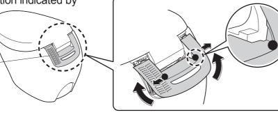
Pull the hand lever to where it stops. (about 30 seconds). • The water surface in the bowl rises.
