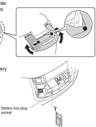
· Unplug the battery box, take out the batteries, put the battery box cable inside the bag, and store
