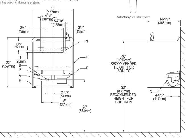
A = Recommended water supply location 3/8" O.D. unplated copper tube connect. Stub out1-1/2" (38mm) from wall shut off by others. B = Recommended waste outlet location. To accommodate 1-1/4" nominal drain. C = 1-1/4" Trap (not furnished).
