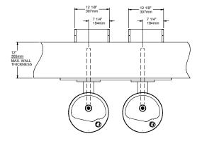
WARNING: The freeze-resistant box must be installed on an interior heated wall where the temperature does not drop below 50 °F (10°C). The front of the box must have unobstructed air flow. Failure to maintain the interior wall temperature and the inside of the freeze-resistant box above 50 °F (10°C) can result in damage to the box which could result in unrestricted water flow.
