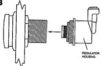
Carefully thread regulator/housing into bottom female thread of push button assembly. Hand tighten.
