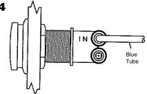
Insert 12" blue tube (included) into regulator part identified as "IN".
