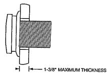
Place push button assembly in 1-1/2" hole. Tighten with hardware.
