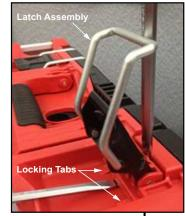
As an aid to removing a damaged Latch Assembly (9), use two large flat blade screwdrivers. Push blades between parts as shown. Twist both screwdrivers at same time to force the blades into opening and work the latch assembly over the two locking tabs.
