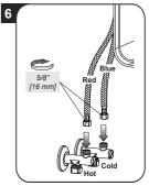
Connect the flexible hoses to the supply connections with rubber gaskets. Secure with wrench. Turn on the water and check for leaks.
