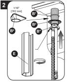
For countertop thicknesses less than 1/16" thick use the rubber gasket (B1) and mounting flange (B2), for all other installations use the rubber gasket (B1) and metal washer (B3).
