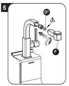
Tighten the shower (F) to the hose interposing the gasket (D3) and confirm the hose can slide smoothly through the passage hole.
