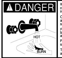
Water temperature over 125°F can cause severe burns instantly or death from scalds.
