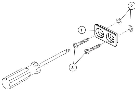
With the mounting bracket (1) oriented as shown, place it over the installed anchors (2) and screws (3). Repeat for second mounting bracket.
