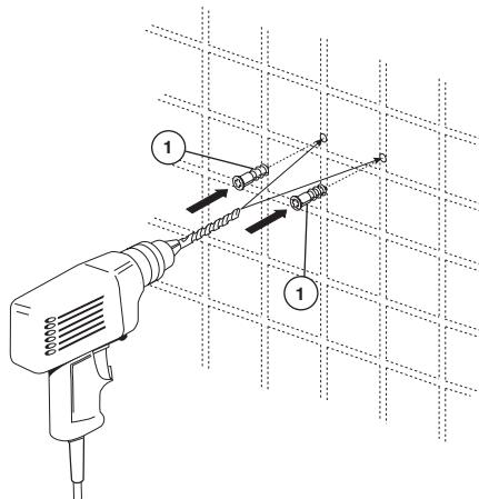
**NOTE:** If possible, it is best to mount at least one end of your tissue holder into a wall stud. Try to locate a wall stud with a stud finder or by tapping on the wall. Place mounting bracket (1) in the desired location. Ensure the mounting bracket is level; then, mark the position of the holes (2) on the wall. Repeat for the 2nd mounting bracket as noted above.
