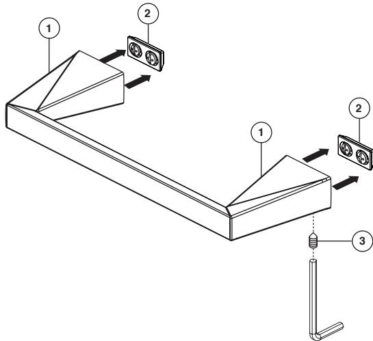
Position body (1) over mounting bracket (2) and tighten set screw (3). Repeat for second mounting bracket. (Set screw should be on the bottom of body)
