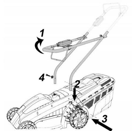
2. Insert the lower handle into the slot (2).
