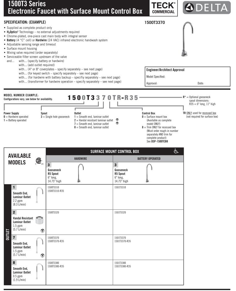
Refer to www.specselect.com for individual models. Batteries included on all battery models. Flow Rates are at 60 PSI. Note: Use these pages as product submittal sheets.
