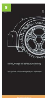
Take your robot close to your WI-FI box for initial setting. Make sure your robot is turned on. ► Press "Add equipment".
