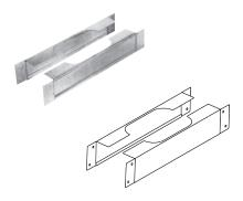
• The firestop spacers center vent in 16"O.C. stud space and serve as a firestop at the ceiling level. This is a required component for Type B 2 x 4 and multi-story Type BW installations.
