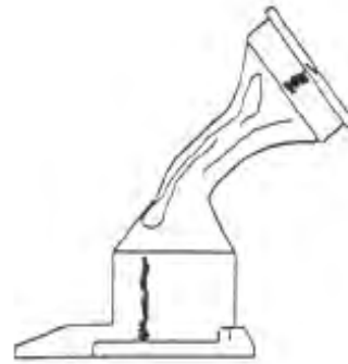
Fig. A-11 Door Handle W/Tab After Grinding
