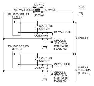
FIG. 1 WIRING DIAGRAM
