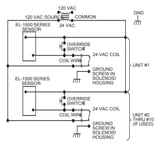
FIG. 1 WIRING DIAGRAM
