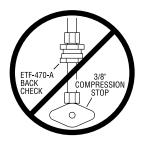
When installing the faucet please, disregard "Step 1 — Install Back Checks." Instead, simply connect the Hot and Cold water supplies directly from the Supply Stops to the Bak-Chek Tee.
