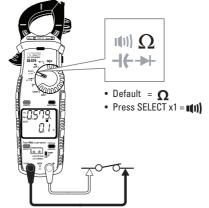
• Buzzer sounds at less than < 40 $\Omega$ .
