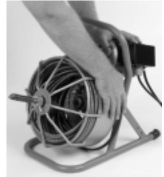
Figure 10 – With belt tension released, slip belt off drum
