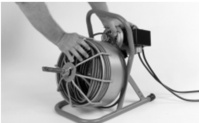
Figure 5 – Push down on motor, slip belt over drum.
