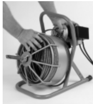
Figure 9 – Push down on motor to release spring tension on belt
