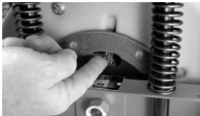
Figure 12 – Lift release pin UPWARD to release drum lock mechanism.
