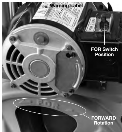
Figure 8 – Proper Drum Rotation (FOR Switch Position)
