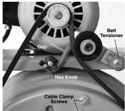
Figure 17 – Torque Limiter Adjustment. (Shown With Belt Guard Removed)
