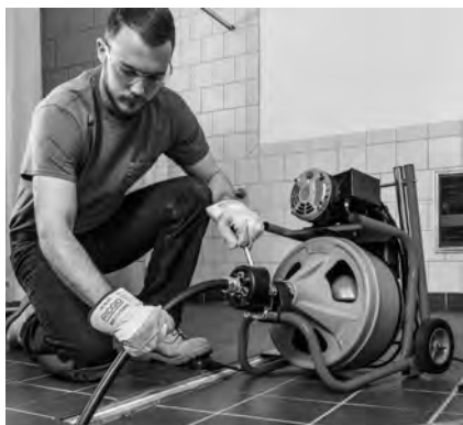
Figure 16 – Using Machine with Guide Hose
