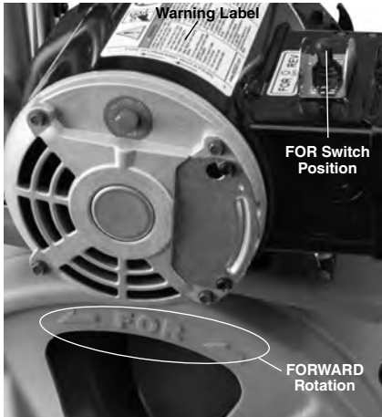
Figure 8 – Proper Drum Rotation (FOR Switch Position)
