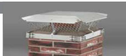
Hood is made from 18 gauge diamond embossed aluminum. Braces 5/8" x 3/4" extruded aluminum. 16 gauge aluminum expanded metal mesh. Band is 2 3/4" - 18 gauge diamond embossed aluminum. Nuts and bolts are stainless steel.
