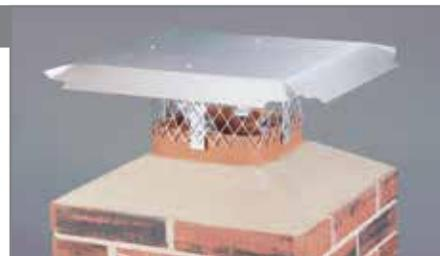
Hood is made from 18 gauge diamond embossed aluminum. Bracing and clamps are 1/2" x 1" extruded aluminum bar. 16 gauge aluminum expanded metal mesh. Nuts and bolts are stainless steel.
