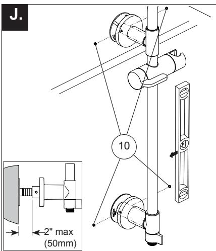
**J.** Note: The lower mounting post may be exposed up to 2" (50mm) from finished wall and lower post of shower column. The escutcheon will cover this area.
