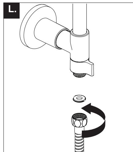
**L.** Ensure the gasket is inserted into the hexagonal hose nut.
