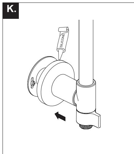
**K.** Apply silicone sealant to the inner groove located on the reverse side of the upper and lower escutcheons.
