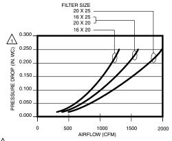
1\ \text{WHEN FIRST INSTALLED. PRESSURE DROP INCREASES AS FILTER BECOMES LOADED. REPLACE FILTER WHEN PRESSURE DROP REACHES 0.5 IN. WC. (0.1 kPa).
