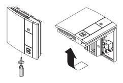
Make the connections using solderless connectors for copper wires. The thermostat wires are non-polarized; this means either wire can be connected to either terminal.
