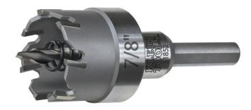
The 7/8-Inch Carbide Hole Cutter is ideal for installing 1/2-Inch conduit and pipe. It features a split-point pilot drill bit to help prevent walking. An integrated flange prevents cutting beyond the sheet metal.
