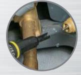
Schrader™ and core removal combination bits for installation/ removal of common TR-4 Schrader™ valves
