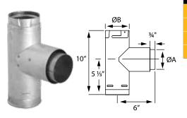
Use for a 90° offset. Attaches directly to appliance as an adapter. Removable twist-lock Clean-Out Tee Cap.
