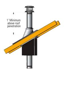
The following design recommendations are a general guideline to assist in the design and selection of venting components for your installation. Always follow DuraVent Installation instructions before installing your chimney system (found with the cap or support box). Installation instructions can be viewed online at www.duravent.com, under Catalogs and Instructions.
