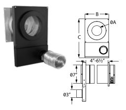
Includes Wall Thimble, Channel Adapter, Flex and 2" to a direct vent for bringing outside air for combustion through an adjustable air channel in wall thimble to appliance without cutting a second hole into the wall. Minimizes down drafts in below-grade installations. Patent-pending.
