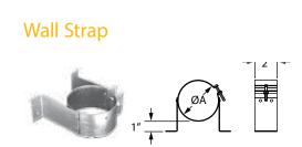
Use to support vent pipe or tee sections. Provides 1" clearance.
