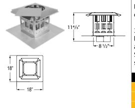
Use when installing a pellet insert into a multi-fuel pellet stove. This termination cap supplies both fresh air and vents exhaust. Lid pivots open for cleaning with three Removable screws and one rivet. Flex sold separately.
