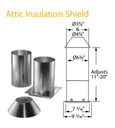
Required for installations that pass through an attic to prevent insulation and debris from accumulating near the vent. Provides 1" clearance to combustibles.
