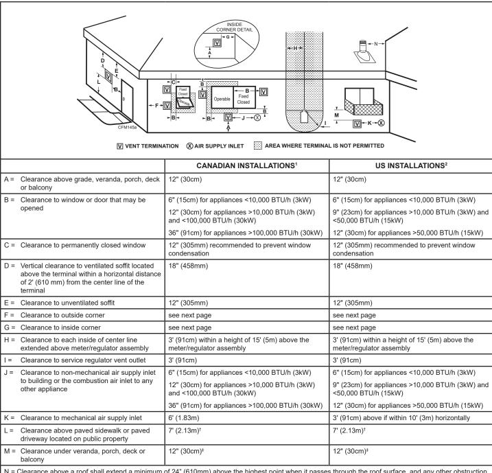
N = Clearance above a roof shall extend a minimum of 24" (610mm) above the highest point when it passes through the roof surface, and any other obstruction within a horizontal distance of 18" (450mm).
