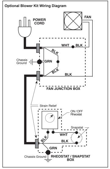
Figure 6.2 - Fan circuit.
