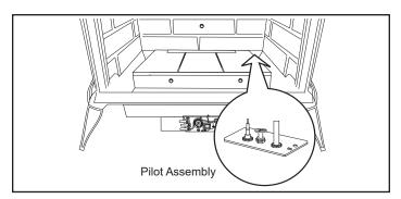
Figure 4.1 - Pilot Assembly location.
