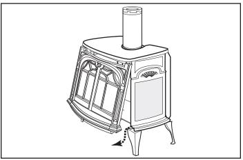
Figure 3.24 - Remove the safety barrier and stove front.
