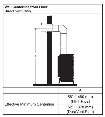
Figure 2.5 - Minimum wall centerline.
