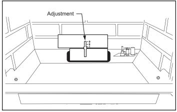
Figure 2.9 - Loosen screw to adjust restrictor plate.
