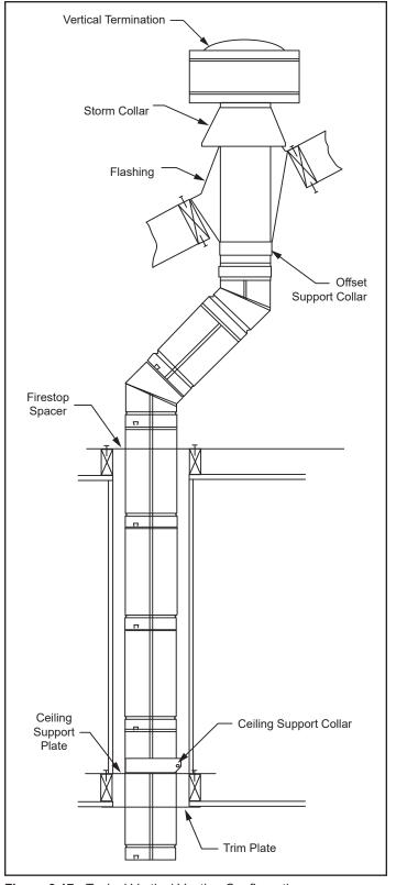
Figure 3.17 - Typical Vertical Venting Configuration
