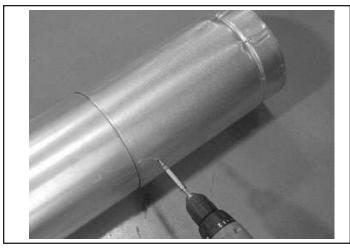
Figure 3.5 - Screws into Slip Section
