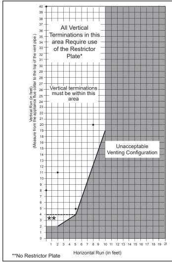
Figure 2.8 - Vertical vent termination window.
