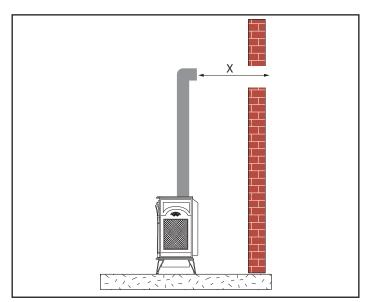
Figure 3.13 - Horizontal Length Requirement
