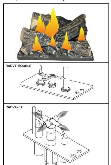
Figure 4.6 - Correct pilot and burner flame appearance.
