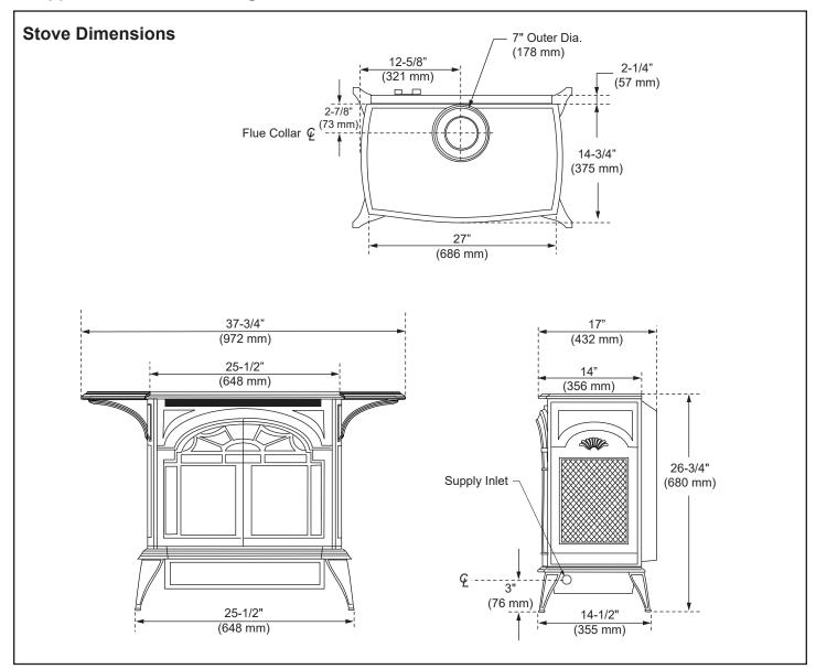
Figure 2.1 - Stardance dimensions. Weight: Fully assembled; 202 lbs.
