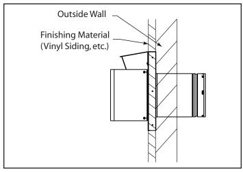
Figure 3.1 - Termination cap on wall
