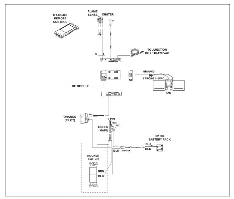
Figure 6.3 - SDDVT-IFT Wiring Diagram
