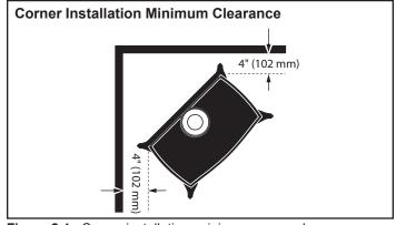
Figure 2.4 - Corner installation, minimum corner clearances.
