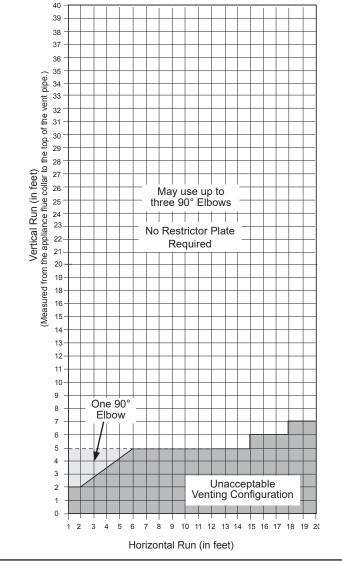
**Figure 2.7** - Horizontal vent termination window.
