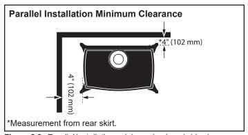
Figure 2.3 - Parallel installation, minimum back and side clearances.
