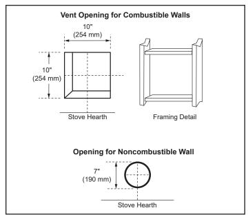
Figure 3.11 - Locate vent opening on wall.
