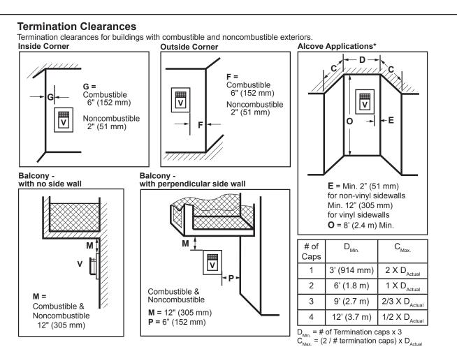
\*NOTE: Termination in an alcove space (spaces open only on one side and with an overhang) is permitted with the dimensions specified for vinyl or non-vinyl siding and soffits.
