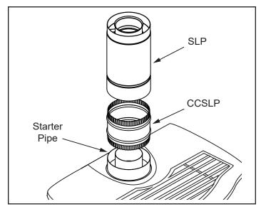
Figure 3.2 - Attach inner assembly to flue collar.
