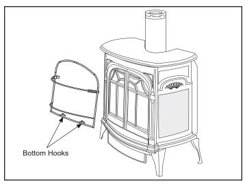
Figure 3.32 - Install safety barrier screen.
