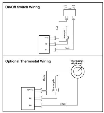
Figure 6.1 - On/off switch and optional thermostat circuit.
