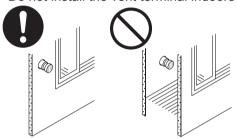
Do not cover the vent terminal with any type of protective screen or enclosure. Blocked terminals can cause abnormal combustion resulting in undesired performance from the water heater.
