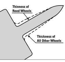
more easily and leave less burr. Also, because of their higher quality, certified material, only Reed wheels can be heat-treated for the perfect balance between hardness and toughness to make the wheels resist breakage and last longer.
