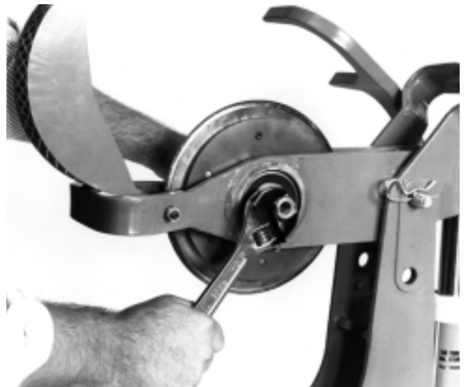
Figure 11 – Remove Locking Nut
