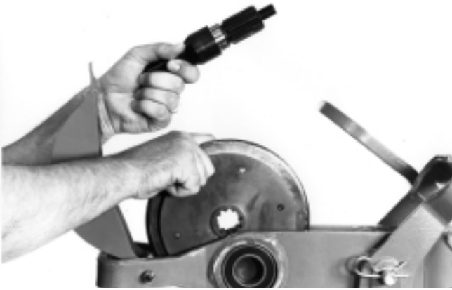
Figure 12 – Remove Cutter Wheel Assembly
