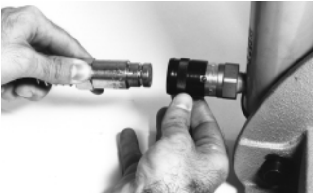
Figure 3 – Connecting Hydraulic Foot Pump to Cutter
