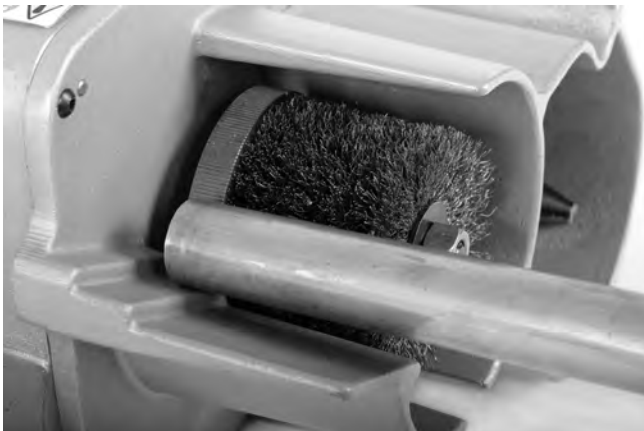
Figure 12 – Deburring O.D. Of Tube
