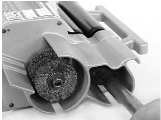
Figure 13 – Reaming I.D. of Tube
