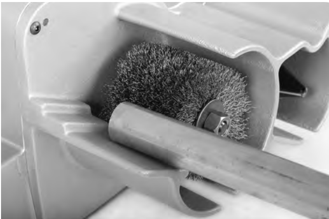
Figure 11 – Cleaning Tube O.D.
