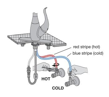
Step 6 Flush supply lines and check for leaks
