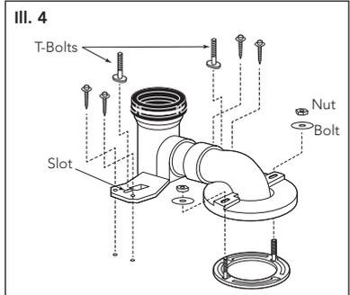
**NOTE:** Level the PVC outlet. Do not use excessive force.
