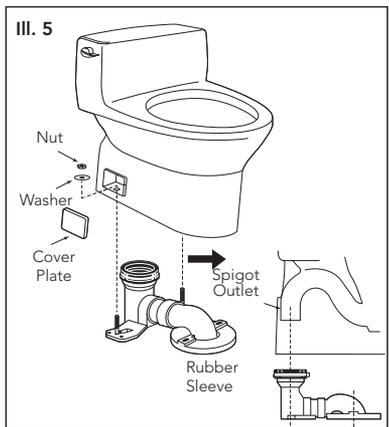
**WARNING!** Do not over-tighten the nuts. Damage to china or plastic parts may result.
