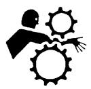
clothing should become caught in the machine, it could continue to wind up, pulling you into the machine. Because the machine has high torque, the clothing itself can bind around your arm or other body parts with enough force to crush or break bones.
