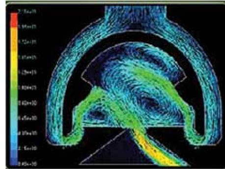
Water expands and collapses inside the H<sub>2</sub>O Chip created high-frequency oscillating streams which allow for distance of throw using 1/3 less flow.
