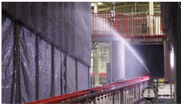
Extensive testing for T5 nozzle efficiency was performed using SPACE calculations
